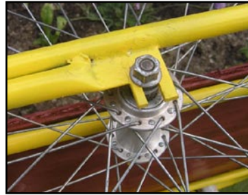
Connection of bottom pulling arm to left-side dropout
