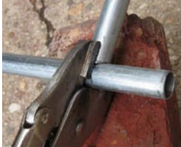
Hold the main frame together for brazing
