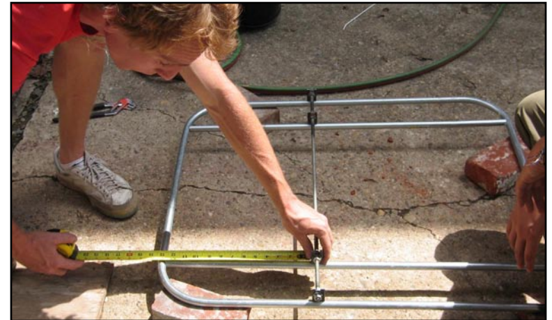
Jake places the dropout jig 13" forward from the back of the mainframe.
