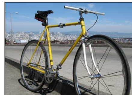
azuki bean: my 2-speed break-away bike frame for travel. the coupling plates are 1/4" flat stock with two 1/4" bolts.
