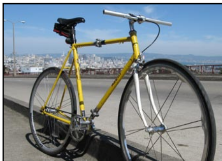
azuki bean: my 2-speed break-away bike frame for travel. the coupling plates are 1/4" flat stock with two 1/4" bolts.
