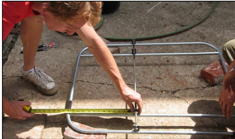
Jake places the dropout jig 13" forward from the back of the mainframe.
