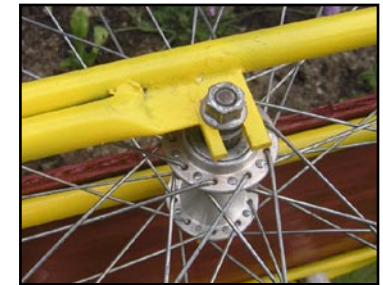
Connection of bottom pulling arm to left-side dropout
