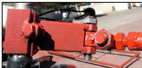
Above: The hitch and U-joint, made from nuts and bolts.
