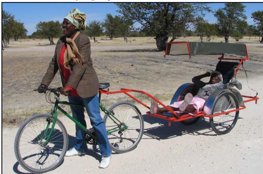
This bicycle ambulance is in use by Ombome Oto HIV/AIDS Home Based Care volunteers in Oshandi, Ohangwena region in Namibia. These health care workers use bicycles to reach their patients in the rural areas, and when further medical attention is required but other traditional or motorized transport is unavailable, they transport their patients on the bicycle ambulances.
