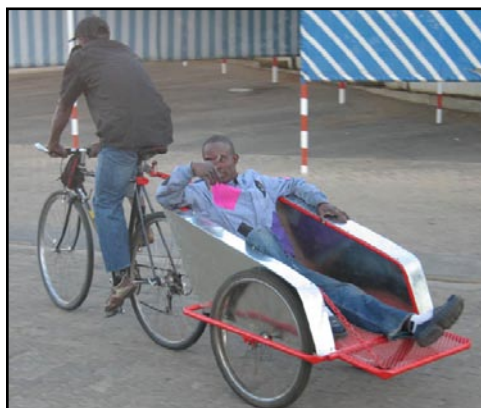
Right: The Bike Bakki, similar to the "chariot model" is designed for manufacture and use in Namibia for transport of goods, water, firewood, and passengers. Lolo is getting a lift from Tate Eliaser, the bicycle ambulance fabricator at BEN Namibia.
