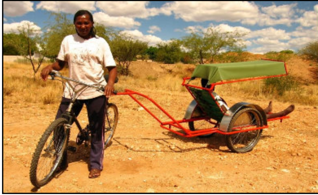
The production model of the BEN Namibia Bicycle Ambulance has wide tyres, a removable and adjustable stretcher, a handle for pulling by bicycle or hand, and a sun shade.
